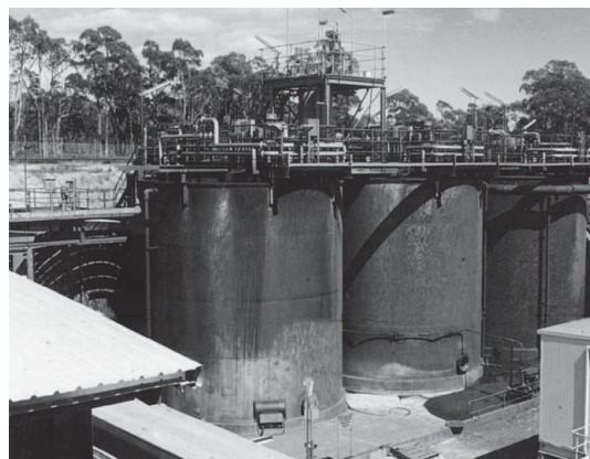
図 2. Tank biooxidation of refractory gold (source: BioMineWiki). Process conditions (e.g. aeration, temperature, pH, reagent concentration, dissolved oxygen) can be controlled in order to achieve required leaching efficiency.
