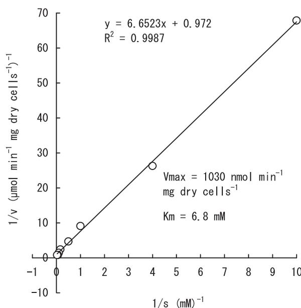
Fig. 8. Determination of  $V_{\text{max}}$  and  $K_m$  on MTBE degradation by *Mycobacterium duvalii* TA5.
