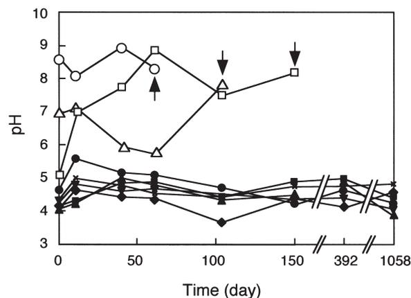
Fig. 3. Comparisons of compost pH and durations of different AHTC systems. An identical composition and amount of garbage, from a feeding facility for school lunch, was subjected to the conventional systems<sup>3,6</sup> from three different commercial sources (maximum capacity, 1 kg/day; indicated by ○, □, and △) and six, identical, independent acidulocomposting systems (maximum capacity, 1 kg/day; indicated by ●, ■, ▲, ◆, ▼, and ×). The composting stopped at the time indicated by arrows.
