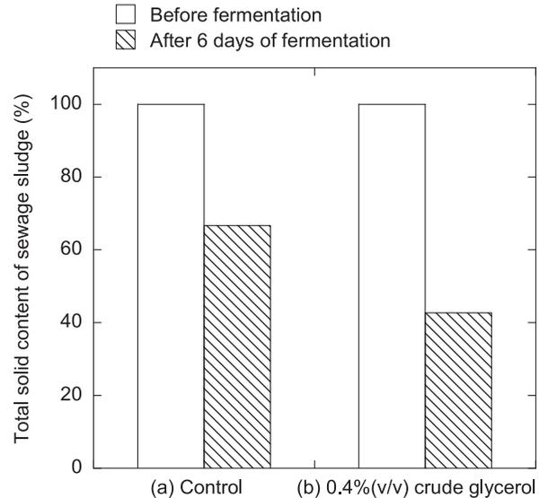
Fig. 4. (a) TS content in sewage sludge from the anaerobic digestion of sewage sludge after 6 days of incubation. Sewage sludge contained 20.4 g/L TS.
