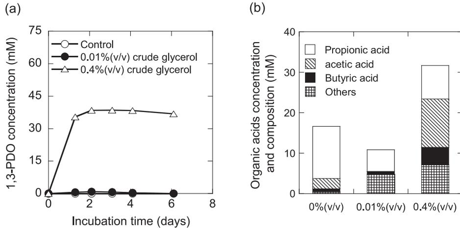
Fig. 2. (a) 1,3-PDO concentration in the fermentation broth from the anaerobic co-digestion of sewage sludge with different concentrations of crude glycerol.
