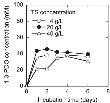
Fig. 3. 1,3-PDO concentration in the fermentation broth from the anaerobic co-digestion of different TS concentrations of sewage sludge with 0.4% (v/v) crude glycerol.
